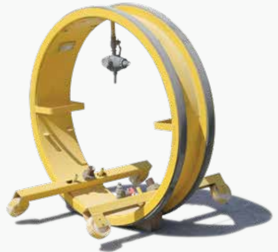
Fig 18 Testing device for the single joints
